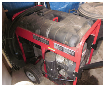
Generac generator, Robin Subarau eng., 10,000 watt
